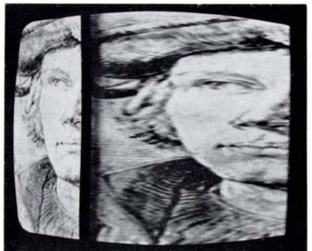
Fig. 17. Television picture illustrating time-axis conversion. The original picture on the left was written line by line into a bucket-brigade shift register and read out at a lower frequency, giving the picture on the right.
