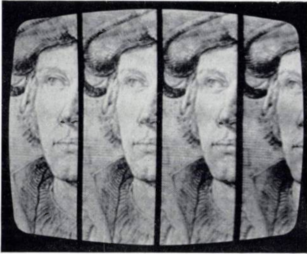
Fig. 13. Photograph of television picture illustrating the low distortion caused by the passage of the same signal through a bucket-brigade delay line. The original picture appears on the left; in the second strip it has been delayed by four integrated circuits of the type shown in fig. 12 (a total of 288 stages). In the third strip the signal has passed through eight of these circuits, and in the fourth strip twelve. It can be seen that there is very little degradation of the picture.
