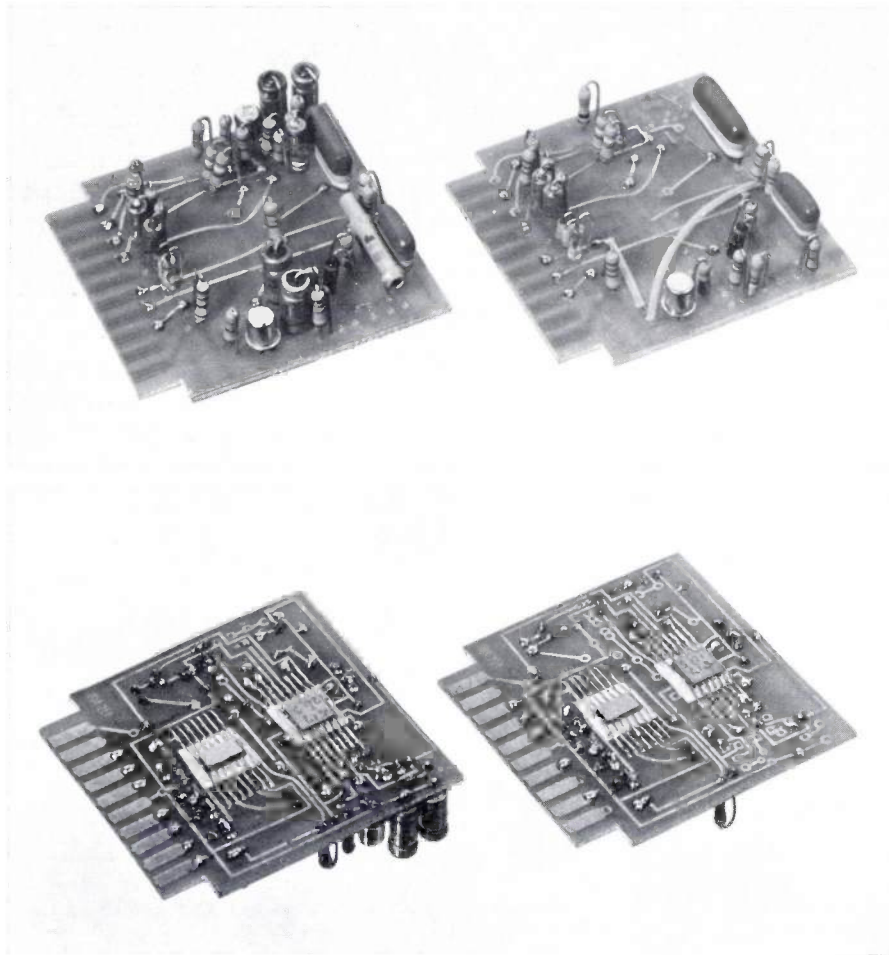
Fig. 21. Practical circuit of a coder ( left ) and a decoder unit ( right ) for DCDM corresponding to the block diagrams in fig. 19. Except for the integrating circuits and one or two discrete components the units are made in integrated-circuit form; only two different types of chip are required.
