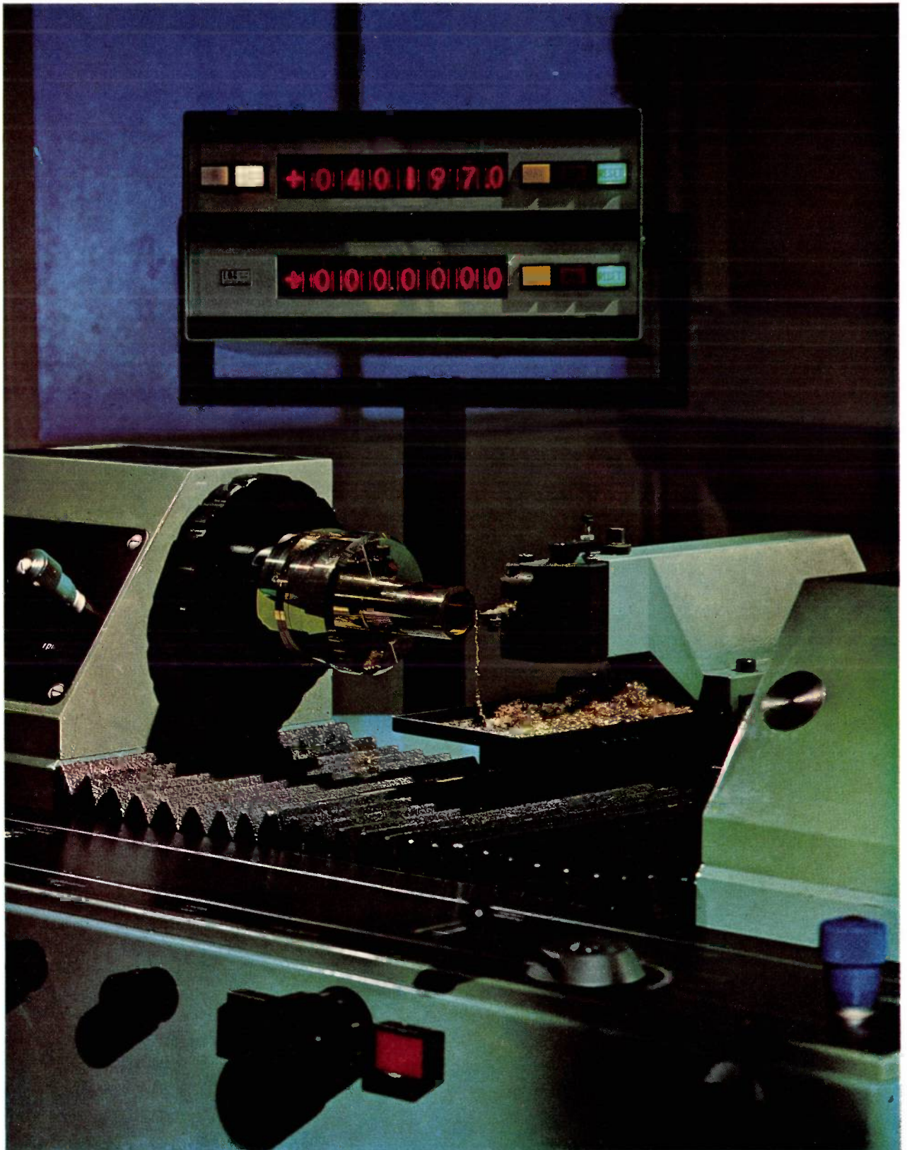
Hydraulically driven precision lathe with hydrostatic bearings for the main spindle and for the carriages, designed in the Philips Research Laboratories. The two numeric displays above the lathe show the coordinates of the cutting tool in ten-thousandths of a millimetre. Machine tools are the subject of the article on the adjoining page.
