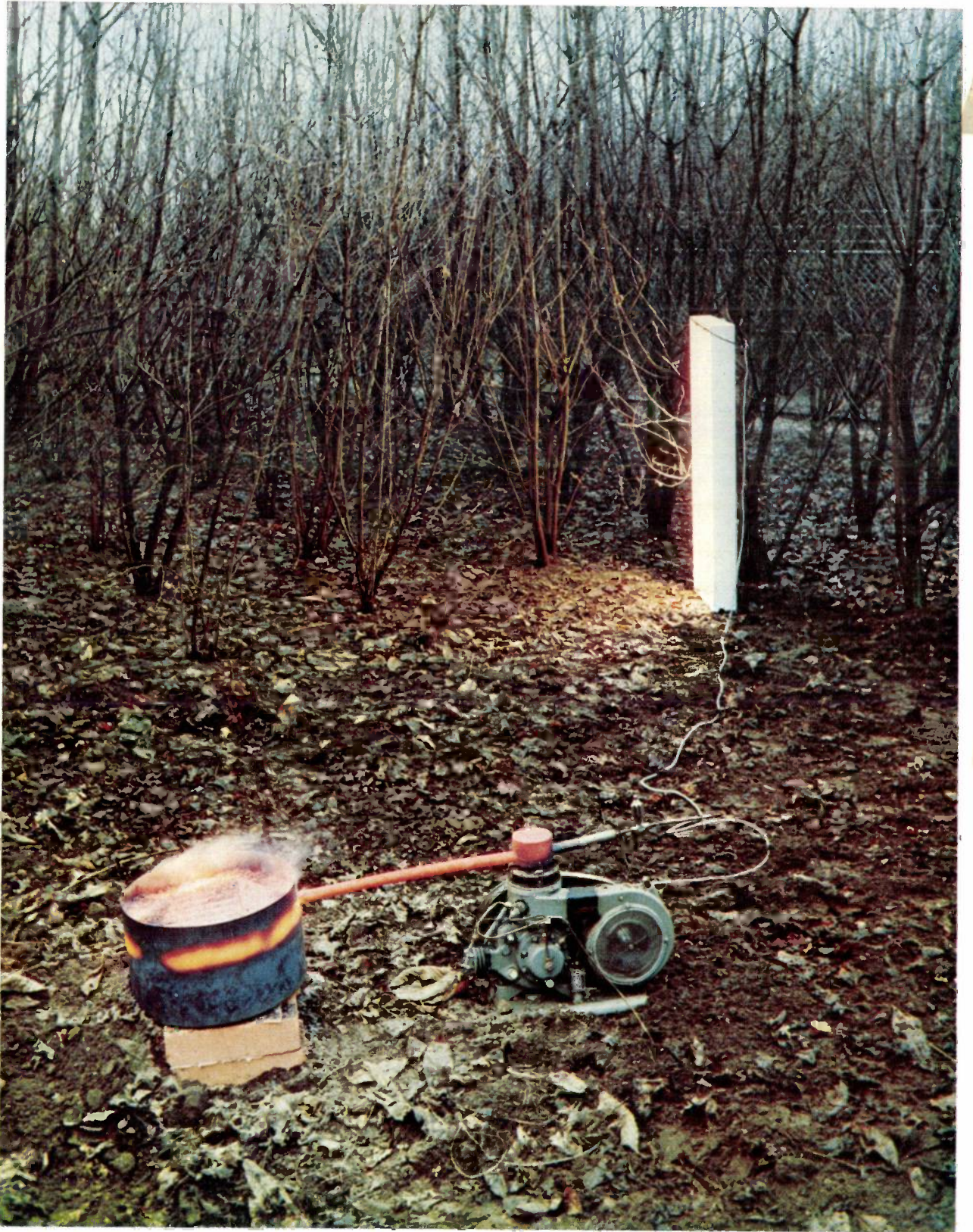
A small generator-set with a Stirling engine driven by the heat from a brazier. The Stirling engine is connected to the heat source by a heat pipe. This method of heat transmission is of considerable interest for vehicle engines.
