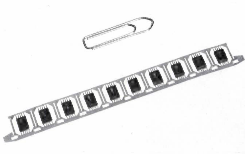
Fig. 3. The integrated Hall circuit in a plastic encapsulation. Tapered recesses at both ends contain pole pieces for increasing the magnetic flux density in the device. In the motor that we have developed this is about 0.6 T ( 1 \text{ T} = 10^4 \text{ gauss} ). The devices are made in strip form and later punched out.
